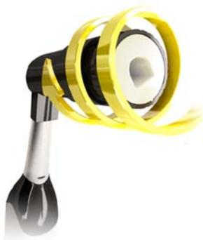
5. Turn the screw counter-clockwise until you reach the next latching point.
