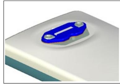
**IMPORTANT!** The elastomeric strip must be seated squarely in the slot for the Sensor to function.
