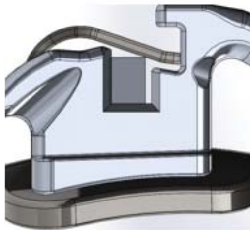
Figure 3: Clip resting on active archwire (0.019" x 0.025").
