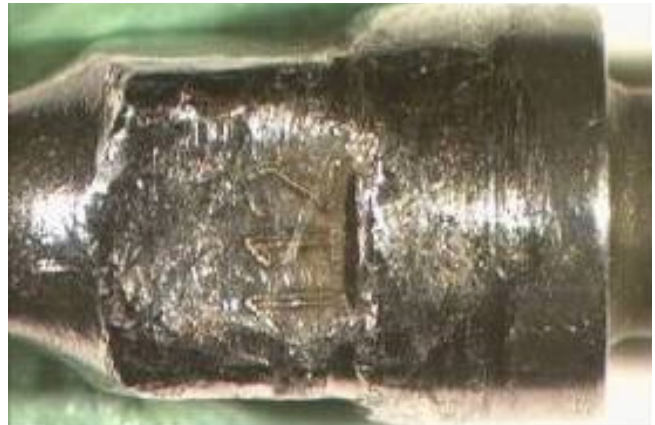
Picture 7 - Damaged four corner shaft
