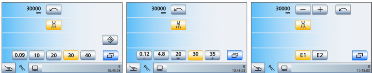
Motor screen with fixed quick setting keys (left), programmable quick setting keys (center) and function levels (right)
