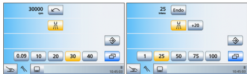
Motor program (speed) and ultrasonic program (intensity) with static quick setting keys
