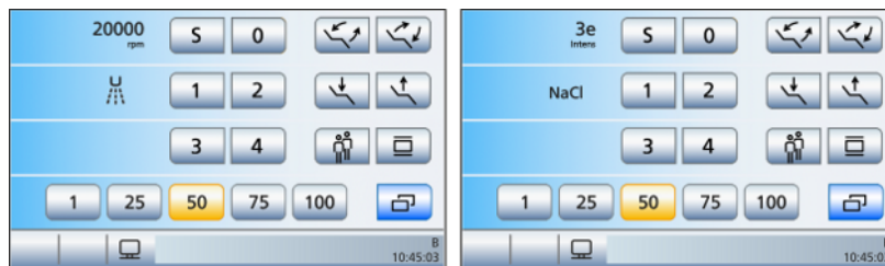
The EasyMode Start programs with instrument functions for motor and ultrasonic (active endodontic function)
