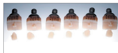
6. Single crowns milled from CEREC Tessera™. The blanks selected were MT blanks (medium translucency).
