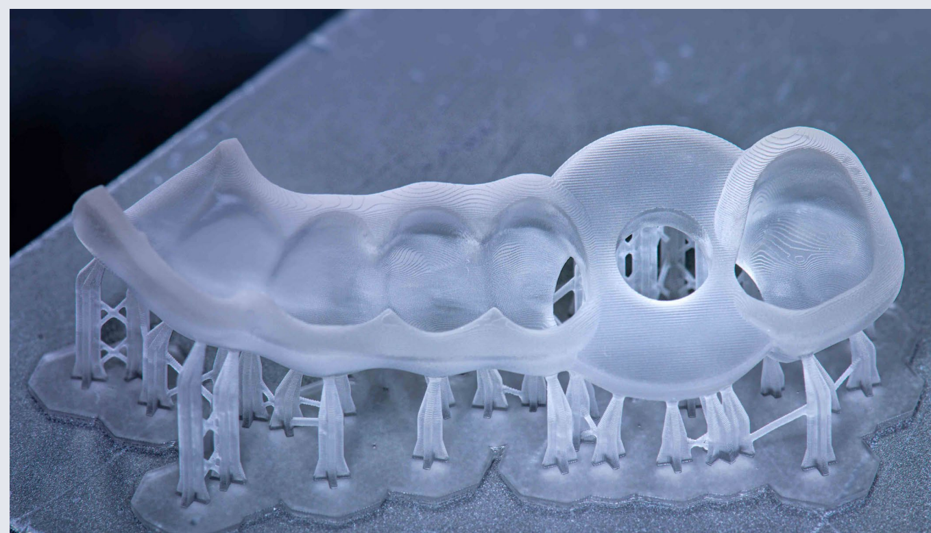
CEREC Guide after 3D printing using Primeprint and post-processing in the Primeprint PPU.
