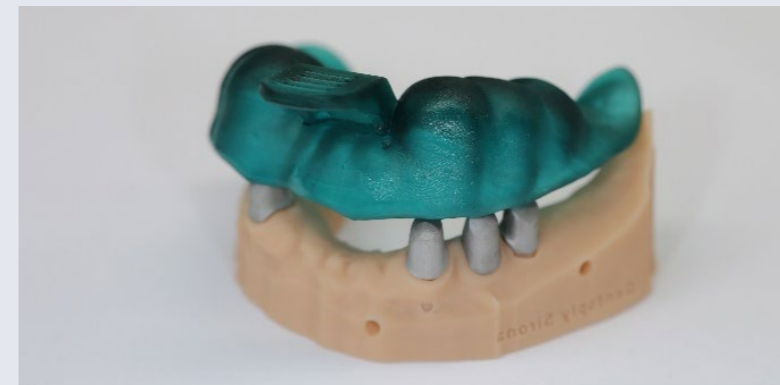
Usage: 3D-printed impression tray on a 3D-printed model, printed with Primeprint Tray and Primeprint Model material
