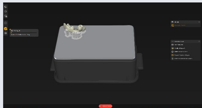
Fig. 6: Splint positioned on Primeprint build plate with supports
