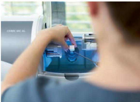
The restoration created on the computer is subsequently milled from a ceramic block.
