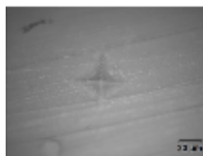
Indentation after firing at 760 °C for 2 min.* Surface is smoothed and hairline fractures are sealed.
