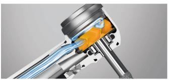
The brake ensures that the idling speed of a dental turbine is limited without noticeably reducing its power.
