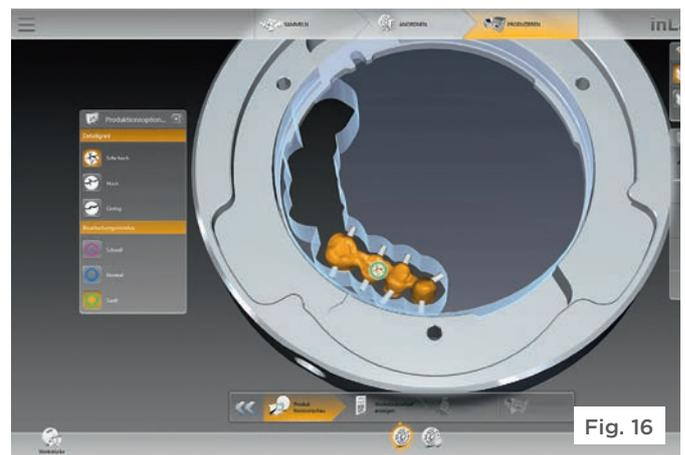
In the production preview, the sprue connections were reduced and the milling job passed on to the laboratory's own inLab MC X5 5-axis milling unit (Fig. 16).
