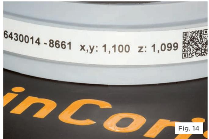
In the current version of the CAM software, the inCoris CCB blank can easily be identified by QR code detected by a webcam (Fig. 14) — a convenient feature that can also be used for all other inCoris blanks. The QR code provides all of the necessary information on the current blank without the inconvenience of manual data entry; the software even recognizes already partially milled blanks.
