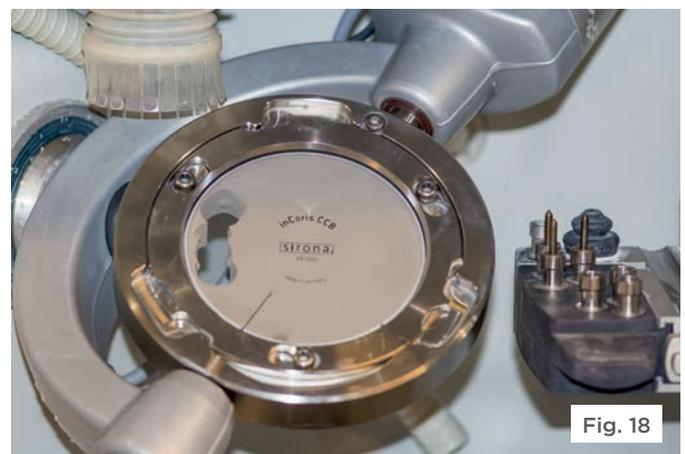
The software presents a reminder screen at this point (Fig. 17) to ensure that both the correct workpiece and the corresponding tool magazine are loaded into the unit (Fig. 18).
