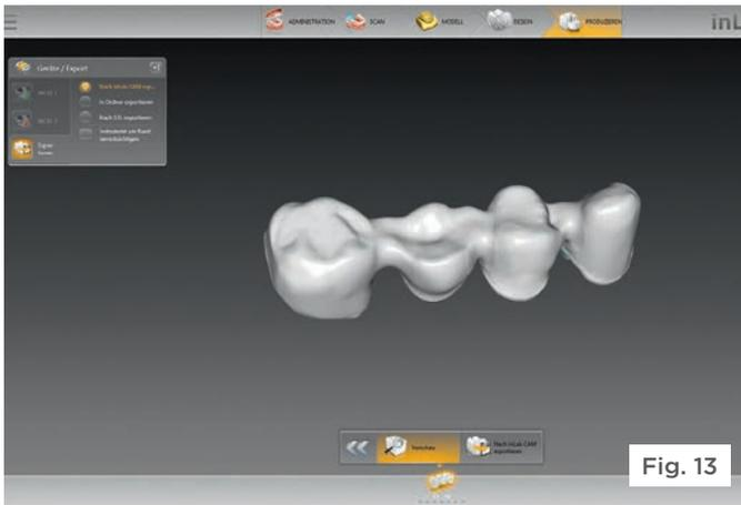
The final check was performed on the preview screen (Fig. 13), from where the data was exported to the inLab CAM 16.0 software.
