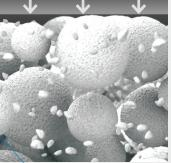
The micro-granulated structure of SphereTEC™ filler is able to bind more free resin compared to usual fillers. Therefore TPH Spectra® ST composite does not stick to hand instruments.
