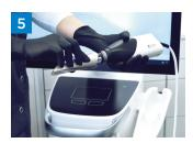
Carefully re-attach the steel sleeve until it locks in place.
