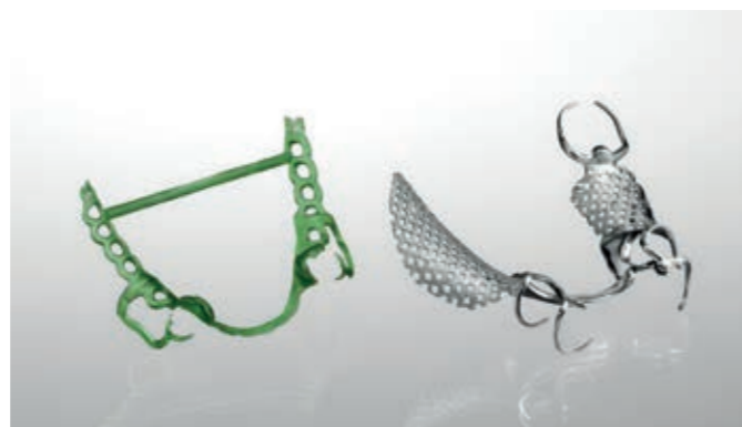
STL export of the design data set*, implementation in wax for subsequent casting or direct production using the laser sintering process (e.g., by inEos X5).
