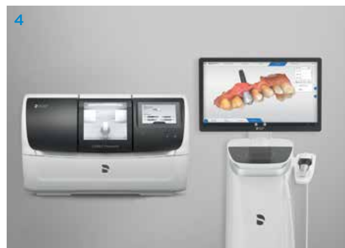
4 Restore: Planning, milling and insertion of the abutment and crown, and capturing and assessing the control images.
