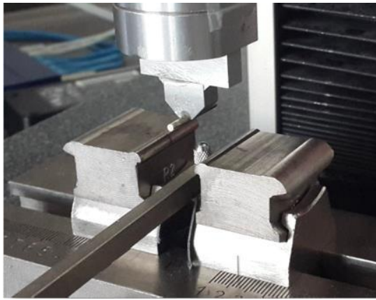
Figure 22 Three-point test set-up with extensometer (Lohbauer U)
