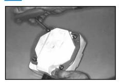
Apply separator to the Dentsply Sirona LabStone, and place the top half of the Flask on the bottom half, <u>ensuring complete, intimate contact and closure of the halves.</u> Secure metal Flask Brackets to the Flask and tighten using a metric wrench, specifically for the Microwave Flask.
