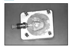
Place the metal Injection Insert into the back of the Flask. Then, slide the plastic Injection Socket into the metal Insert as far as possible.
