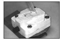
Apply separator (such as sodium silicate or another alginate or petrolatum separator) over pour #2 once set. (A separator plate may be used as an alternative.)
