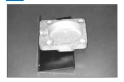
Apply petrolatum to the inside of the Metal Flask, and place the Flask on the Leveler (side "1" up).
